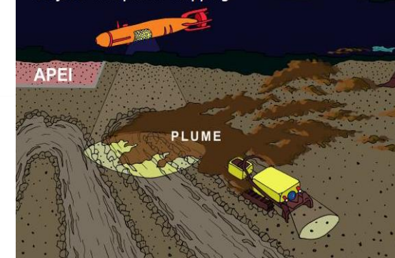
Schematic of a real-time mining monitoring concept, utilizing an autonomous vehicle for seafloor and plume mapping
